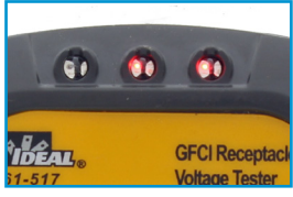
Red Lights Indicate Incorrect Wiring
