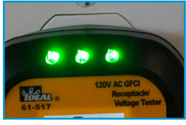
Green Lights Indicate Correct Wiring
