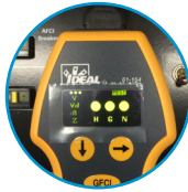
Displays H N G polarity
