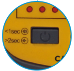
On/Off Button Short Press for On, Long Press to Defeat Audible
